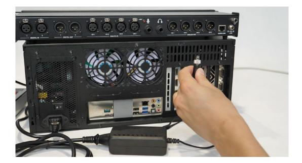
Bolt the locking screw. Picture below.
