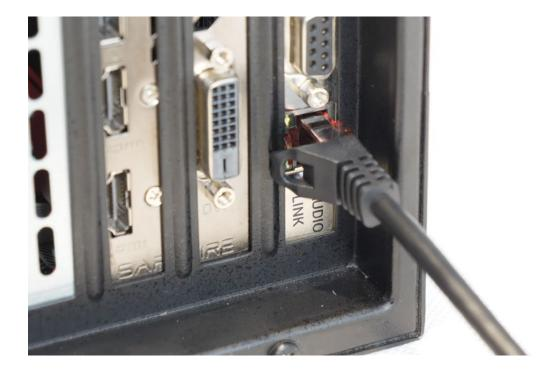
Plug the second end of the cable to the Audio Link Connector in ADB 100. Picture below.
