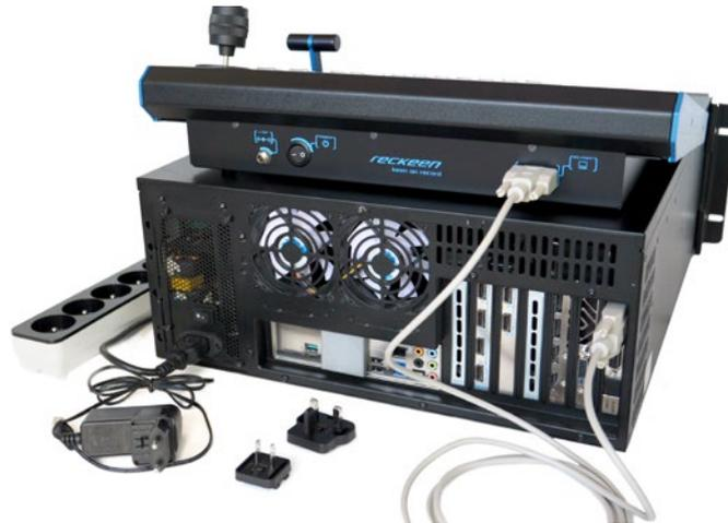
Use a proper power supply adapter used in different types of electrical networks. Select the appropriate adapter and insert it into the power plug. Move it forward until you hear a click. Picture below.
