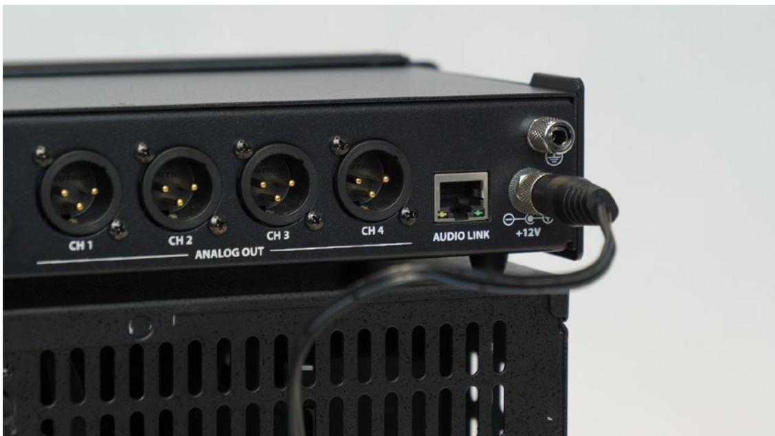
Next connect the power supply unit to the electrical outlet. Picture below.
