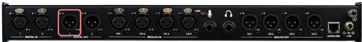
Digital output 2 on the XLR connector. Picture below.
