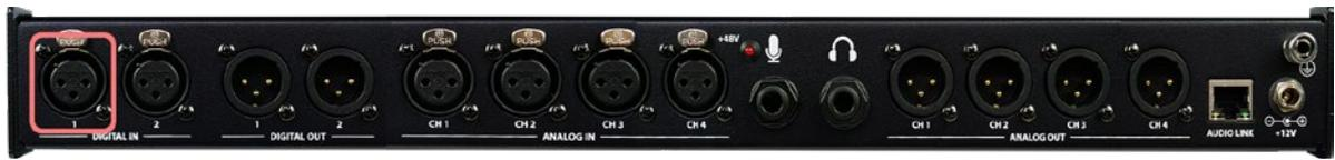
Digital In 2 input on the XLR connector. Picture below.
