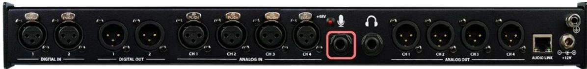
In Configuration Window you can find Microphone settings for the microphone connected to AUDIO BOX panel (ADB -100).Picture below. There are two operating modes: a None mode with a dynamic microphone, for which you can set the Gain value with a slider, and a Phantom mode with a condenser microphone. When you switch to the Phantom mode, you will be warned that a voltage of 48 V will be applied to the speech insert. A red LED lights up on the ADB 100.
