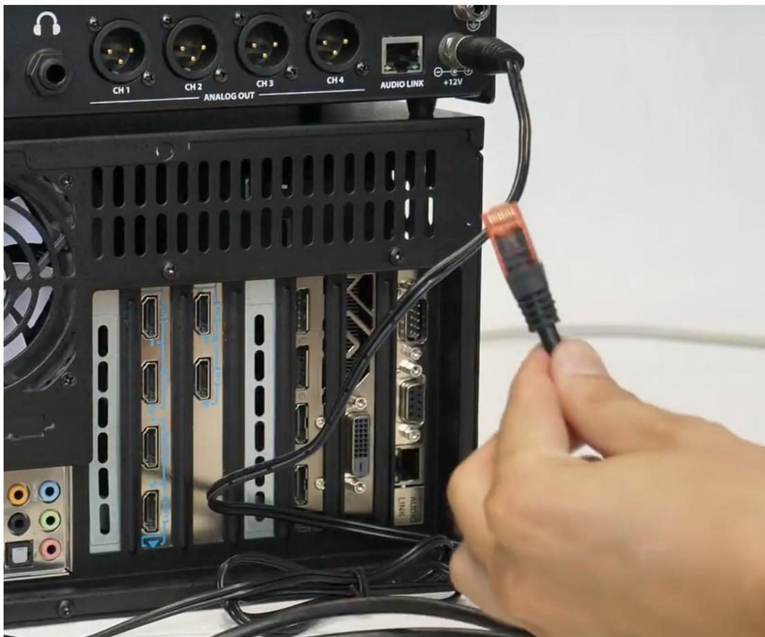
Plug the end of the cable to the input / output card. Picture below.
