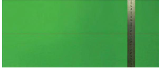
Then check whether the camera is also leveled in the depth. Accuracy cannot exceed 1 mm.
