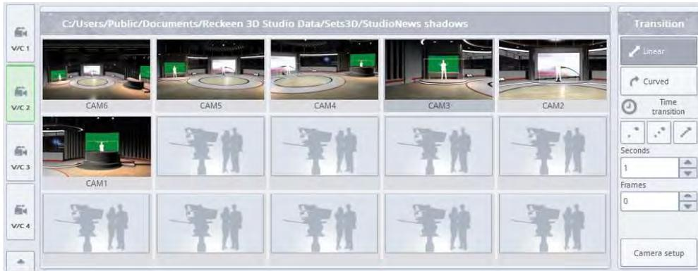
The Reckeen 3D Studio system is equipped with **4 V/C** channels, that is **Virtual Cameras**.
