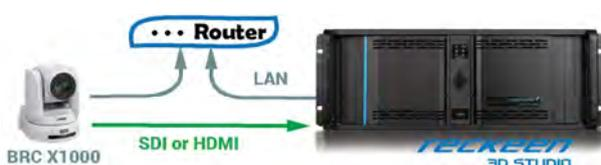
Another reason for red-coloured button might be that the HDMI or SDI video connection was disconnected between the PTZ camera and the Reckeen system or LAN ports connection has been interrupted.
