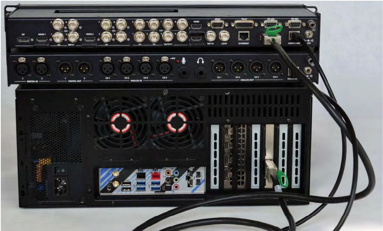
The next step is to connect the RS232 port to the VKey100 control panel
