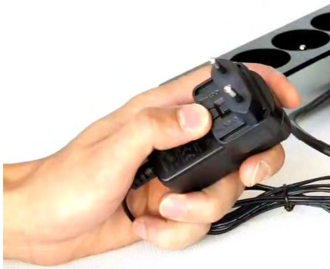
First connect the power supply plug to the VKey 100 / 200 keyboard power socket and bolt the locking screw. Picture below.
