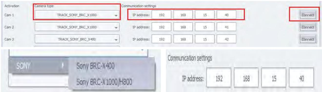
If all cable connections are correct and the camera's IP address is correct, we can press the connect button to connect the camera with the application. Press the **Connect button**:
