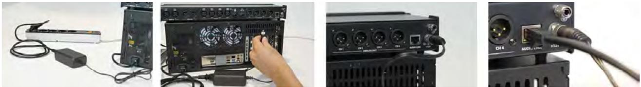
After connecting the power supply to all devices - these devices should signal the power supply via red Reckeen LEDs.
