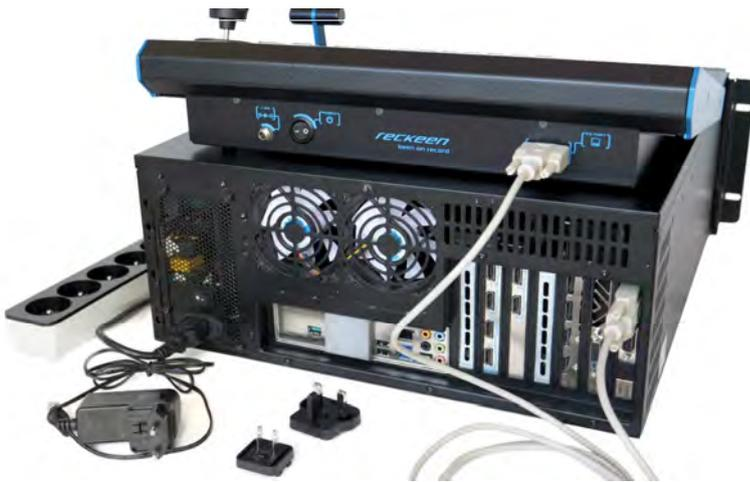
Connect the keyboard to the system using RS 232 communication cable with DB9 connector. Plug the end of the cable to the input / output card. Connect the other end of the cable to the keyboard's port. Screw in the locking screws. Picture below.
