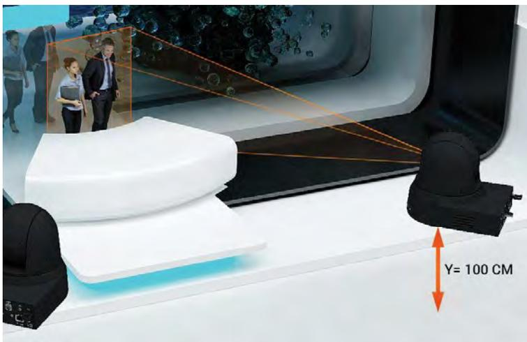
Under "**Y Positions**" input a distance from the floor to the PTZ camera's base. This distance needs to be measured in centimetres.
