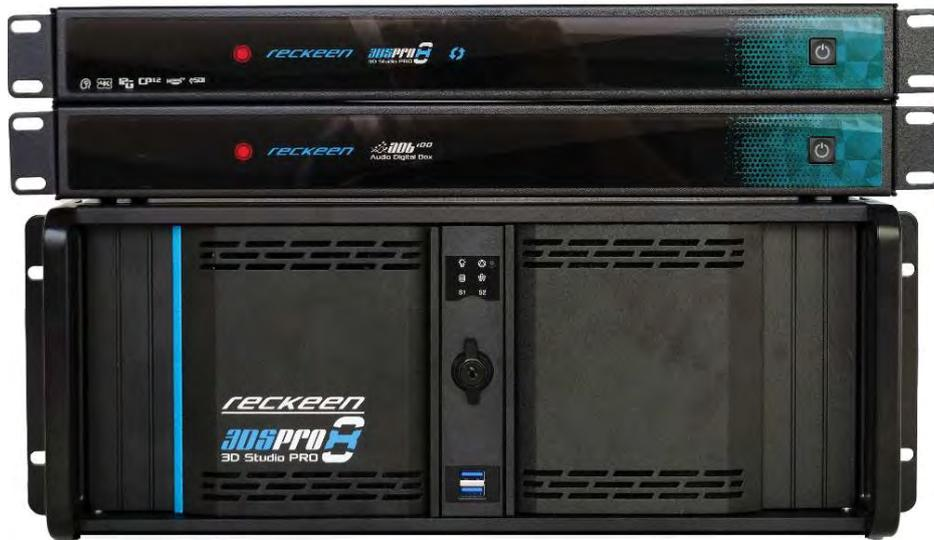
Reckeen 3DSPRO and 3DSPRO X8 Studio System is housed in 19" 4U Rackmount chassis.
