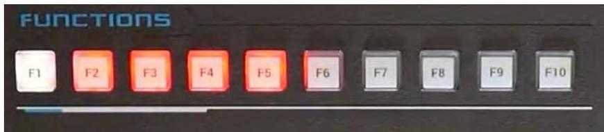
The second test is JOYSTICK's calibration. Move it to the right and to the left to its extreme positions. When it's completed, the F2 LED will light up in white. Picture below.
